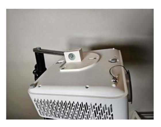
Cameras are mounted and calibrated before shipping, one camera for reading the shot, the second is for the barrel analyzing tool (optional)
